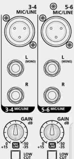
**STEREO LINE INPUT (Ch. 3/4 - Ch. 5/6)** Plug in your keyboard, line level or stereo devices here. Gain scale +15 dB/-35 dB (Ch. 3/4 - Ch. 5/6). The corresponding channel works as a mono channel when MIC input 3/4 or 5/6 is used.
