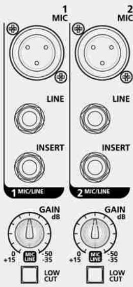
**MIC input (Ch. 1 - Ch. 5/6)** Connect your microphones to these balanced XLR connectors: pin1=Earth, pin2=Hot, pin3=Cold. These inputs are provided with +48 V phantom power for condenser or electret microphones. Gain scale 0 dB/-50 dB.
