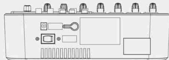
AC IN SOCKET for External Power Supply 18 V AC – 1000 mA.
