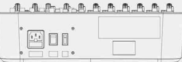
**VDE AC IN SOCKET** AC VDE socket to connect the mixer to AC power supply.
