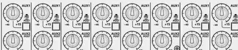
**PRE/POST button:** When released, the signal is extracted in pre-fader position (independently from the fader level); when pressed, the signal is extracted from post-fader position (the send level depends on the fader level).
