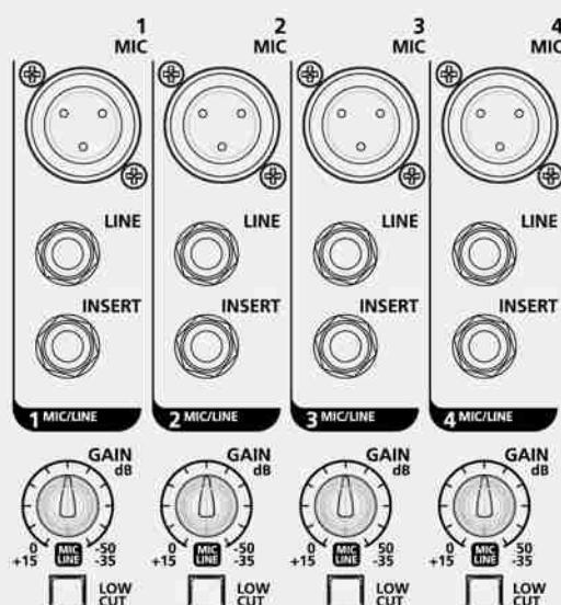
**LINE input (Ch. 1 - Ch. 4)** Connect your line level devices to these TRS jack connectors: tip=Hot, ring=Cold, sleeve=Earth. These inputs are suitable for external pre-amplifier and DI-boxes. Gain scale +15 dB/-35 dB.
