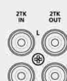
**2TK IN - 2TK OUT.** These unbalanced RCA connectors are suitable for connecting audio player and recorder devices.
