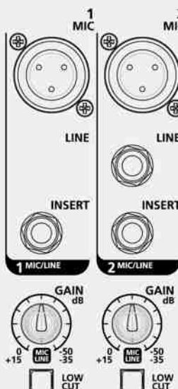
**MIC input.** (Ch. 1 - Ch. 5/6) Connect your microphones to these balanced XLR connectors: pin1=Earth, pin2=Hot, pin3=Cold. These inputs are provided with +48 V phantom power for condenser or electret microphones. Gain scale 0 dB/-50 dB.
