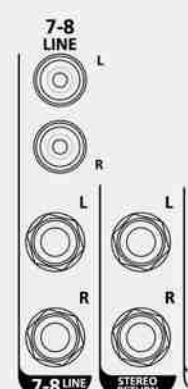
**RCA LINE INPUT.** (Ch. 7/8). Plug in your low-level or consumer devices, like CD players, computers or mobile phones here (adapter needed). LINE INPUT Ch. 7/8 is replicated also with 1/4 inch. Jack.
