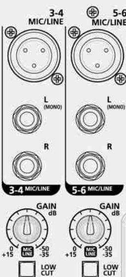
**STEREO LINE INPUT.** (Ch. 3/4 - Ch. 5/6). Plug in your keyboard, line level or stereo devices here. Gain scale +15 dB/-35 dB (Ch. 3/4 - Ch. 5/6). The corresponding channel works as a mono channel when MIC input 3/4 or 5/6 is used.
